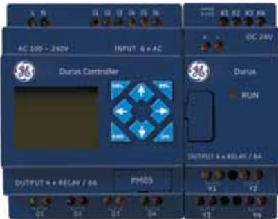
The Durus Controller can be programmed using both the built-in display and keypad or with the Durus Controls Software. The software provides convenient program creation and editing. Programs can be saved on a
