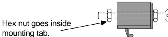
**Figure 2-1. Mounting Tab Assembly**
