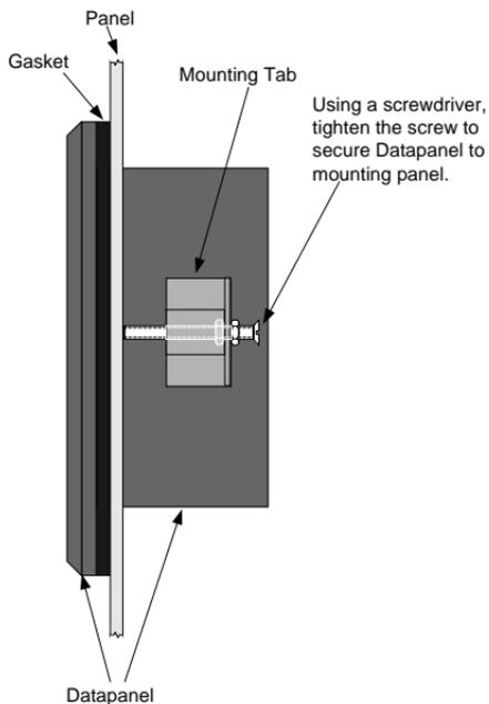
**Figure 2-3. Securing Datapanel, Side View**
