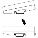
The CPU and connecting carriers must be installed on the same section of 35mm x 7.5mm DIN rail, 1mm thick. Steel DIN rail is recommended. The DIN rail must be electrically grounded to provide EMC protection. The rail must have a conductive (unpainted) corrosion-resistant finish. DIN rails compliant with DIN EN50032 are preferred.
