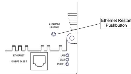
The Ethernet Restart pushbutton has two functions:
