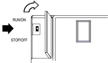
If Run/Stop mode switch operation is enabled, the switch can be used to place the CPU in Run mode.
