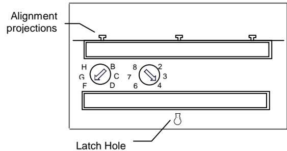
Press the module straight down onto the carrier, seating it fully.
