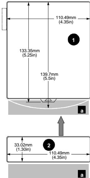
Carriers must be mounted on a horizontal DIN rail.
