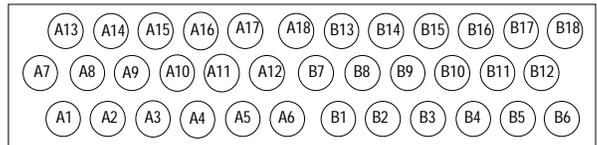
The carrier accommodates current levels up to 2 Amps per point or 8 Amps per each power and ground, and a voltage range of up to 264 VAC. Voltage transients up to 300 VAC will not damage the carrier.
