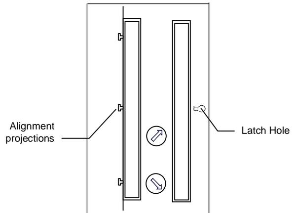
Press the module straight down onto the carrier, seating it fully.
