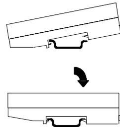
All connecting carriers must be installed on the same section of 35mm x 7.5mm DIN rail. The rail must have a conductive (unpainted) finish for proper grounding. For best stability, the DIN rail should be installed on a panel using screws spaced approximately 6 inches (5.24cm) apart.
