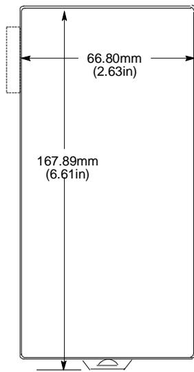
Carriers may be mounted on a horizontal or vertical DIN rail. The carrier with module attached fits into a 70mm deep enclosure. Rated thermal specifications are based on a clearance 2 inches (5.1cm) above and below the equipment and 1 inch (2.54cm) on each side of the assembled equipment. Allow adequate space for I/O wiring.
