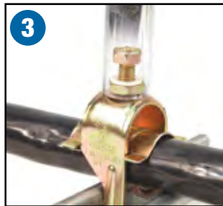
...until it 'blocks' and will no longer turn. Installation is complete. Note: When pre-set torque engages, lock-nut separates from bolt head and stops firmly against clamp body.
