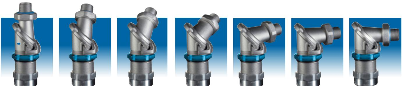
Turn blue compression nut one-half turn to loosen and rotate hub. Tighten blue compression nut to hold hub in place at desired angle.
