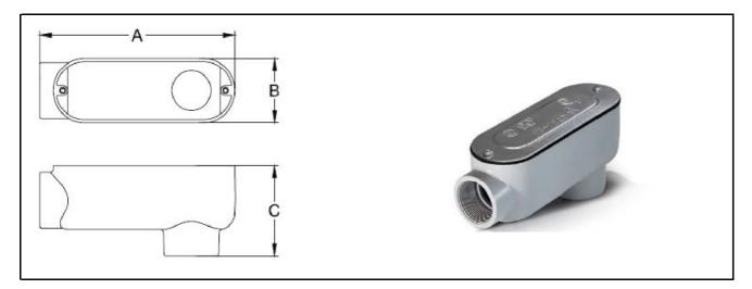
USE: To join Rigid Conduit or IMC and provide access to the interior of the raceway system for wire pulling, maintenance, additions or splicing as permitted by the National Electrical Code. The configuration of threaded entrances and covers permits installation and access from the appropriate direction.
