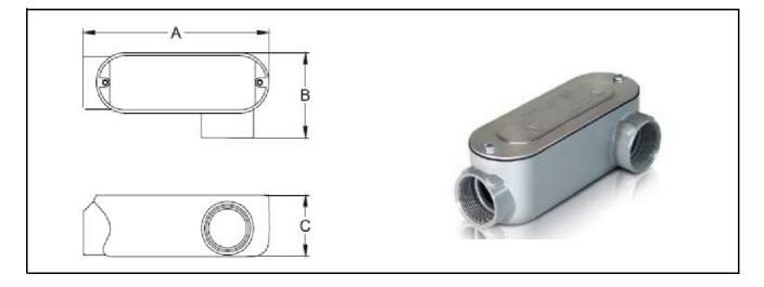
USE: To join Rigid Conduit or IMC and provide access to the interior of the raceway system for wire pulling, maintenance, additions or splicing as permitted by the National Electrical Code. The configuration of threaded entrances and covers permits installation and access from the appropriate direction.
